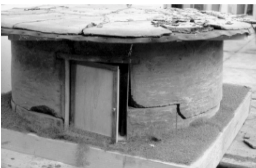
3-4 to 3-8 Earthquake tests with models of square and circular shape (Minke 2001)
